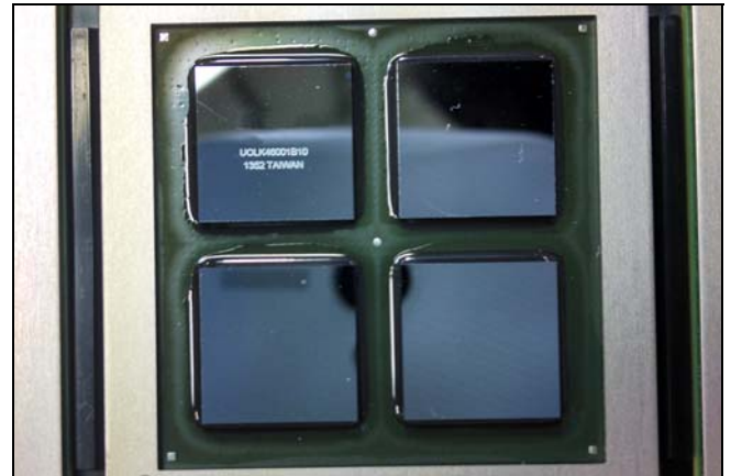
FIGURE 3. A 500W 28nm ASIC mining chip, cooled by a PC water cooling system with a waterblock, pump, custom radiator and external cooling fans.
