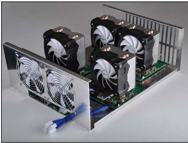
FIGURE 1. A 28nm mining device to be connected to an external power supply.
